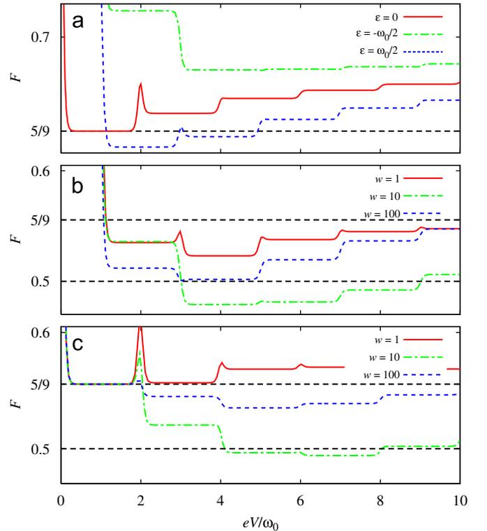
Fig. 1. Fano factor  $F$  as a function of voltage  $V$  (units  $\omega_0/e$ ) for  $\lambda = 1.4$ . (a)  $F$  for  $w = 0$  and different the energies of the level:  $\varepsilon = 0$  (level on-resonance) and  $\varepsilon = \pm\omega_0/2$ . (b)  $F$  at fixed  $\varepsilon = \omega_0/2$  for different values of the relaxation strength  $w$ . (c) Same as in b but for  $\varepsilon = 0$ . In all panels,  $E_c = 10\omega_0$  and  $k_B T = 0.02\omega_0$ .
